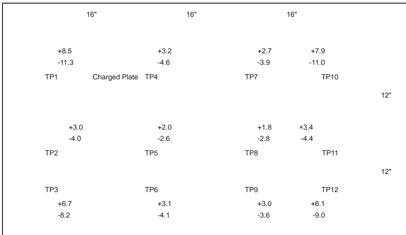
Figure 10. 50665 Neutralization (Discharge) Times at 120VAC, 60Hz input
