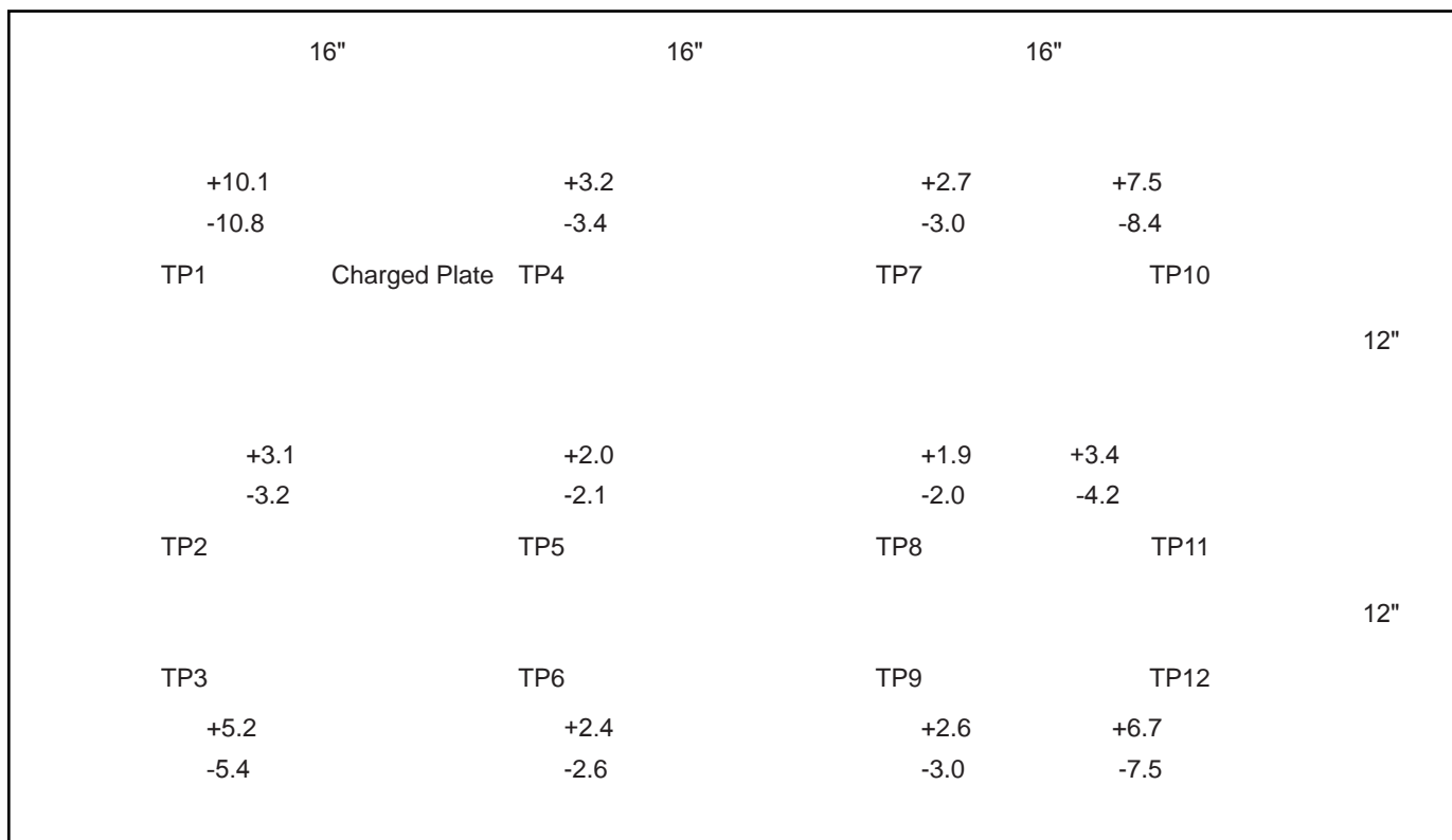
Figure 12. 50672 Neutralization (Discharge) Times at 220VAC, 50Hz input
