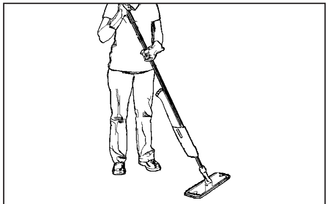
Figure 6. Applying floor finish with Flat Mop (optional).
