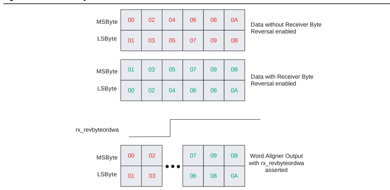
Figure 1-57. Receiver Byte Reversal Feature
