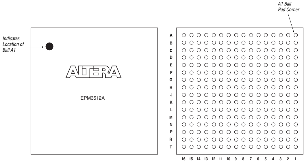
Figure 18. 256-Pin FineLine BGA Package Pin-Out Diagram
