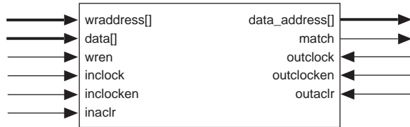
Figure 23. APEX 20KE CAM Block Diagram
