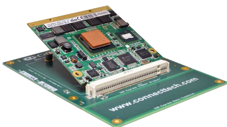
Qseven to COM Express® Adapter with module installed
