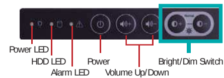
Bright/ Dim Switch for Sunlight Readable Display (optional)
