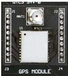
Figure 5: The Development Board GPS Receiver Section
