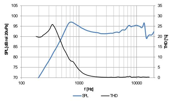
measured in IEC baffle at 700mW in 10 cm distance with 1ccm back cavity
