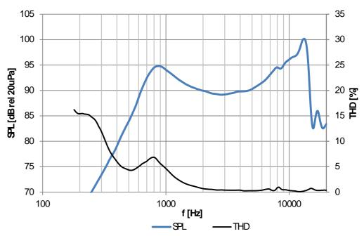
measured in IEC baffle at 350mW in 10 cm distance with 1ccm back cavity
