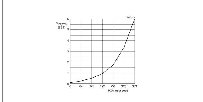
Noise measurement at ADC outputs; coupling capacitor at input is grounded, so only noise contribution of the front-end is evaluated. Front-end works at 18 Mpixels with line of 1024 pixels whose first 40 are used to run CLPOB and the last 40 for CLPDM. Data at the ADC outputs are measured during
