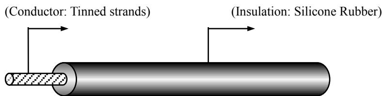
**UL3132 - Silicone Rubber Wire 150°C 300V (22 AWG)**
