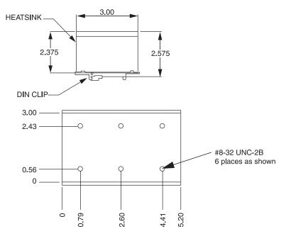
**DIMENSIONS:** inches **TOLERANCES:** ±0.02 inches **MATERIAL:** AISI 6063-T5 Aluminum
