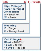
\*Order the relay with the coil voltage in the part number as shown above. The coil voltage will appear on the coil plate near the coil terminals rather than in the P/N on the relay.
