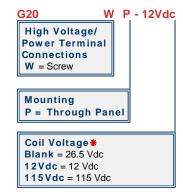
\*Order the relay with the coil voltage in the part number as shown above. The coil voltage will appear on the coil plate near the coil terminals rather than in the P/N on the relay.
