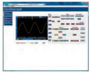
The built-in LAN interface allows you to easily capture screenshots at a user-configurable refresh rate with a web browser. A GUI simulating the front panel provides full DSO control. This feature can be useful in an education setting.
