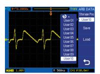
Store user arbitrary waveforms internally (up to 10 waveforms) or externally as an ARB or CSV file to a USB flash drive.
