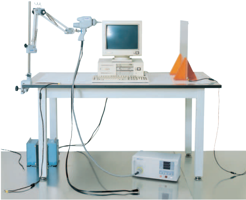
Test set-up example with ESS-801
