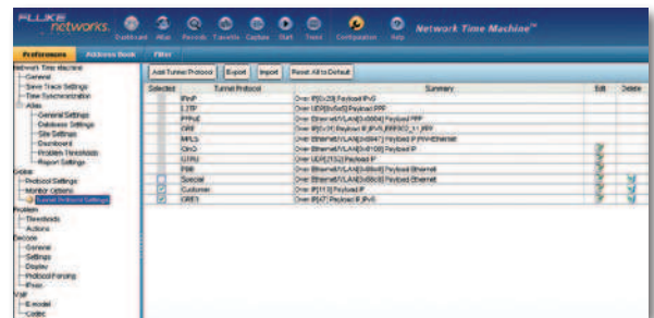
Figure 4. Support for a wide variety of tunneling protocols is provided, or define your own.
