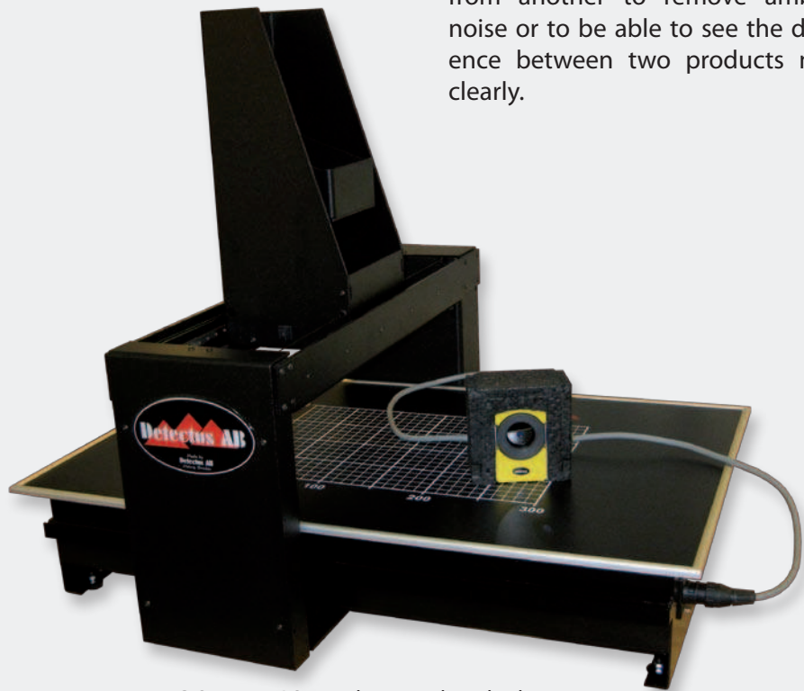
EMC-Scanner RS 321 showing detached heat probe
