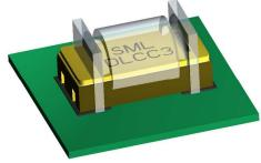
The physical dimensions for the DLCC3 ceramic package are designed to be different from the published dimensions for the "D-5B" and "E-MELF" outlines. The DLCC3 design fully utilises the recommended solder footprint for the "D-5B" / "E-MELF" Package, and as such presents a drop in replacement for existing board designs.
