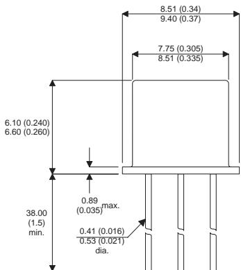
**Bipolar NPN Device in a
