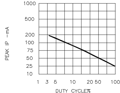
Fig.6 MAX PEAK CURRENT VS. DUTY CYCLE % (REFRESH RATE f = 1\text{kHz} )
