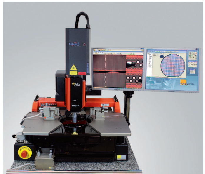
The digital video microscope iVista LC with laser cutter on a PA200 probe system.
