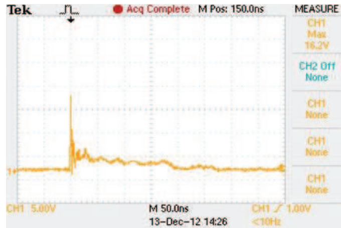
FIGURE 1 8kV POSITIVE ESD CLAMPING WAVEFORM
