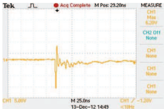
FIGURE 2 8kV NEGATIVE ESD CLAMPING WAVEFORM
