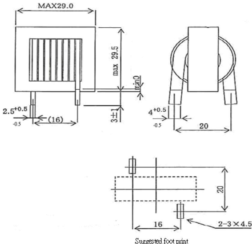
All dimensions are given in millimeters, unless otherwise specified, tolerance  $\pm 0.5$ mm
