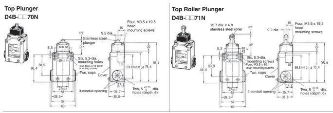
Note: Unless otherwise specified, a tolerance of ±0.4 mm applies to all dimensions.
