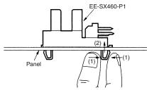
Pressed mounting holes are ideal for mounting the Photomicrosensor. When mounting the Photomicrosensor to a panel that has pressed mounting holes for the Photomicrosensor, be sure to mount the Photomicrosensor on the pressing side of the panel, otherwise it may be difficult to mount the Photomicrosensor and an insertion force of five to six kilograms may be required.
