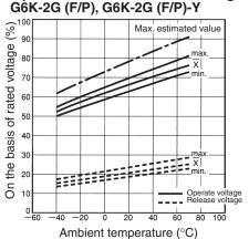
Ambient Temperature vs. Must Set or Must Reset Voltage G6KU-2G (F/P)-Y
