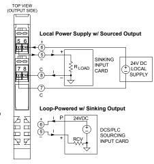
100 ohm Pt RTD or 0-900 ohm input ◆ 4-20mA output (sink/source) ◆ 12-32V DC loop/local power
