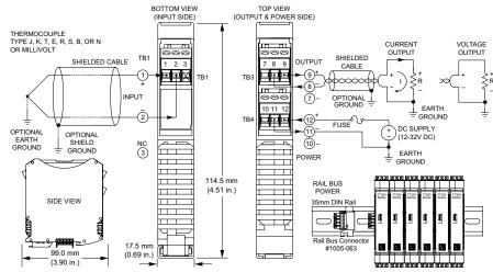
Universal thermocouple/millivolt input ◆ Universal current/voltage output ◆ 12-32V DC local/bus power
