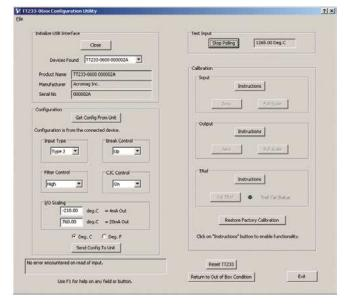
TT233 Model software allows you to configure transmitters offline, save the file, and download settings into units later, at your convenience.
