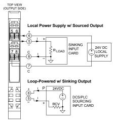
Universal thermocouple or ±100mV input ◆ 4-20mA output (sink/source) ◆ 12-32V DC loop/local power
