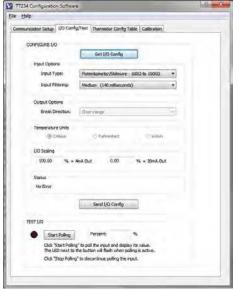
TT234 Model software allows you to configure transmitters offline, save the file, and download into units later, at your convenience.
