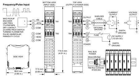
Multi-range frequency/pulse input • Universal current/voltage output • 12-32V DC local/bus power
