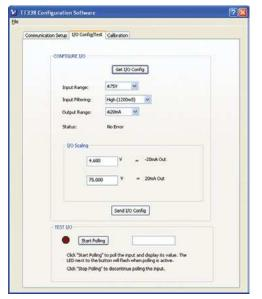
TT338 Model software allows you to configure transmitters offline, save the file, and download into units later, at your convenience.
