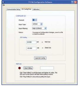
TT236 Model software allows you to configure transmitters offline, save the file, and download into units later, at your convenience.
