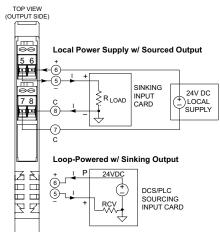
Multi-range ±20mA or ±500mV input ◆ 4-20mA output (sink/source) ◆ 12-32V DC loop/local power
