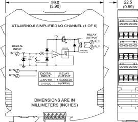
Form A normally open SPST 5A relays • 4-32V logic input 6 discrete input/output channels •
