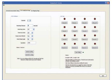
BusWorks XT software (download free from www.acromag.com) allows you to configure transmitters offline with USB, save the file, and download settings into units later, at your convenience.
