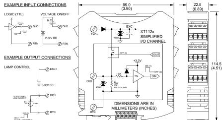
16 discrete tandem input/output channels ◆ Modbus TCP/IP, Ethernet/IP or Profinet communication
