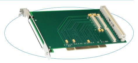
This carrier card converts a PMC module to a PCI board form factor for easy use in a PC-based computer.
