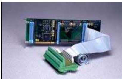
The 5025-552 termination panel and 5025-550 signal cable make field I/O connections to the APC8620 carrier easy.
