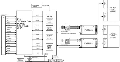
Two Industry Pack mezzanine module slots ◆ Non-Intelligent carrier card ◆ CompactPCI bus interface
