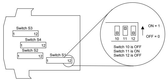
Switch S1 and S2 configure the input type and range, and switch S3 and S4 configure the output types, ranges and a few additional functions. The switch settings are explained in the next few pages. The diagrams refer to switch positions 0 and 1, with 0 being OFF and 1 being ON. This is illustrated in the picture above.
