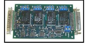
end, allowing the user to expand in multiples of 4 up to the full 16 outputs available on the SDD16. Measuring  $5.6 \times 2.75$  inches (14  $\times 7$  cm) this board is compatible with our SNAPTRACK mounting track. The SDDRB4 can be powered separately on terminal blocks, or on pins 7 and 8, allowing for use of a single power supply for the entire system. A single SDDRB4 requires 200mA at 10 to 16VDC, and 4 boards require 800mA at 12 to 16VDC for all 16 relays.
