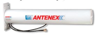
air filled radome yields a higher efficiency and greater performance than the stamped or printed circuit versions. This entire antenna package is 1.6 lbs. and comes with an 18" pigtail of low loss coax cable terminated with an N female connector. The YE series has a VSWR of <2.1:1 from 2.4 GHz to 2.48 GHz and can be mounted outdoors in even the most harsh weather conditions.
