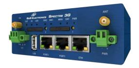
The SPECTRE 3G cellular router connects Ethernet equipment and remote LANs via the cellular telephone network. It creates secure Ethernet connections in locations where cable connections are impractical, as is so often the case with devices like ATM machines and remote video cameras. The SPECTRE 3G also creates reliable mobile Ethernet connections.
