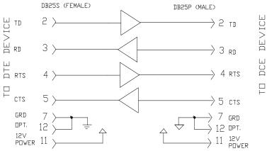
When connecting the Model 232SPOP4 it is recommended that all signals that are outputs be connected. The Model 232SPOP04 derives power from these signals, even if they are not used by your system.
