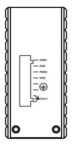
While only one power source is required to power up the media converter, two power sources offer redundancy for those mission critical applications. (PWR1 and PWR2)
