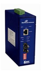
This quick installation guide describes how to install and use the hardened compact Media Converter. Capable of operating at temperature extremes of -40 to +75  $^{\circ}$ C, this is the media converter of choice for harsh environments constrained by space.
