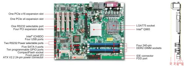
RUBY-9716VG2AR is based upon the Intel® Q965 chipset with five SATA II ports together, one IDE channel and CF socket which is a perfect combination for storage interfaces for kinds of applications; supports Intel® Matrix Storage Technology.
