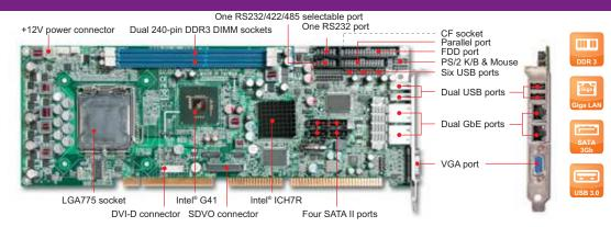
ROBO-8779VG2AR is based on the Intel® G41, ICH7R chipset and supports Core™ 2 Quad sku processors. It supports DDR3 memory up to 4GB. It's the entry level product and suitable for Digital Signage, Kiosk, and Multimedia applications.
