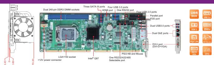
ROBO-8112VG2AR-Q87 is based on Intel Q87 chipset and workstation processor sku like Core i5/i7. Build with flexible PCI express expension, it's suitable for Medical, Industrial automation, and digital signage applications.
