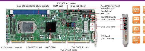
ROBO-8110VG2AR is based upon the Intel® C206 chipset and workstation processor sku like Xeon® and Core™ i3. Built with flexible PCI express expansion, it's suitable for medical, industrial automation, and digital signage applications.
